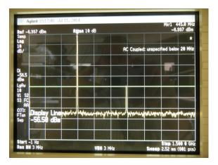
Next, we measured Jim's unit on high power setting at ~444 MHz and ~224 MHz.
