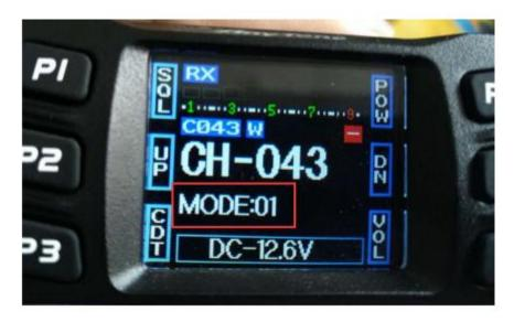
3) Press and hold PTT key on the external speaker mic. MODE no. Change to blue color, then rotate the channel knob to choose the frequency band you need
